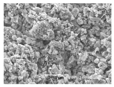
Fig. 6. SEM image of the lime-MK paste at one week cured at 20°C temperature.
