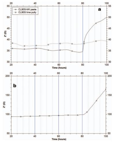
Fig. 5. Bulk resistance as function of time for the test at 20°C (b) and 25°C (a).
