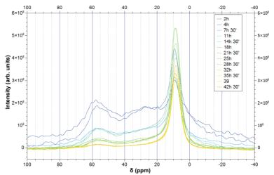
Fig. 12. <sup>27</sup>Al NMR spectra of MK mixed with lime over a period of time of 42 h and 30 minutes at 30°C temperature.
