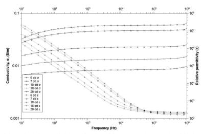
Fig. 3. Conductivity and relative permittivity as function of frequency at 6, 7, 10, 18 and 28 days, for the test at 20°C.
