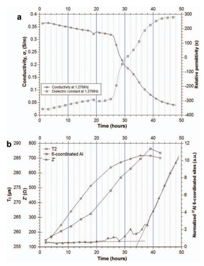
Fig. 11. (a) Changes in conductivity and dielectric constant during the first 48 h of the test at 30°C temperature. Measurement were taken at 1.27 MHz frequency (b) Comparison of the  $T_2$  relaxation time,  $^{27}$ Al MAS NMR spectrum and Z' EIS spectrum.
