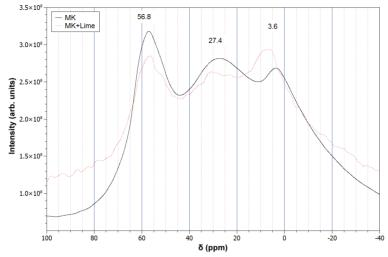
Fig. 1. <sup>27</sup>Al NMR spectra of MK before (continuous line) and after mixing with lime (dashed line).
