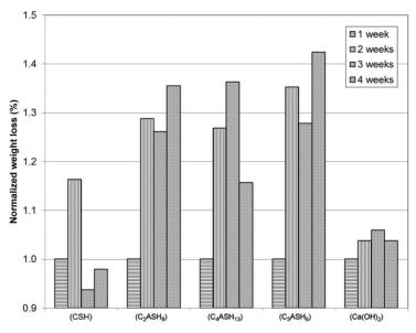
Fig. 8. Change in the amount of different hydraulic compounds formed at 20°C temperature. Calculation in percentage from the thermo-gravimetric analysis, normalized to the value of the first week.
