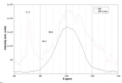
Fig. 2. <sup>29</sup>Si NMR spectra of MK before (continuous line) and after mixing with lime (dashed line).
