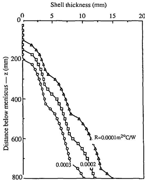
FIGURE 16. Effect of thermal contact resistance  $R$  on the shell thickness on plane  $x=316\text{mm}$ .
