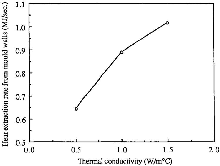
FIGURE 18. Effect of thermal conductivity  $k$  of the mould powder on the overall heat extraction rate from the mould wall.
