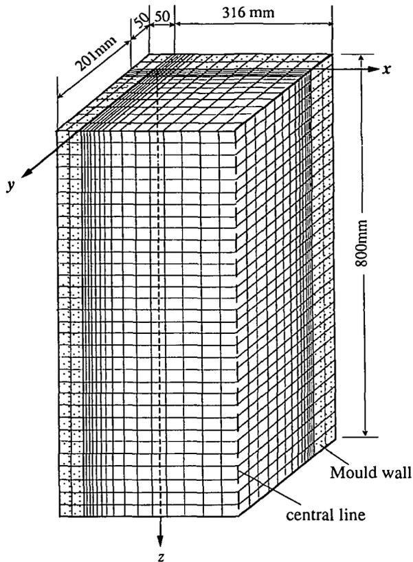
FIGURE 7. Coordinate system, computation region and the grid mesh.
