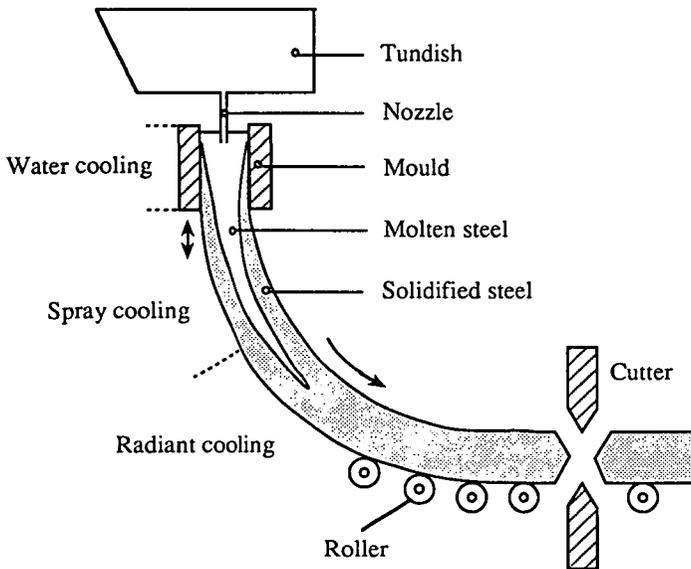
FIGURE 1. The continuous casting process.
