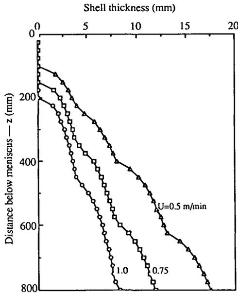
FIGURE 13. Effect of casting speed  $U$  of the steel on the shell thickness on plane  $x=316$ mm.
