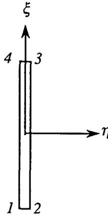
FIGURE 5. A four node thermal contact element.
