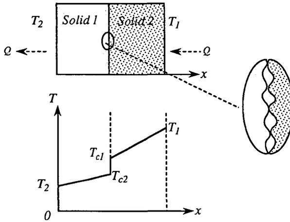
FIGURE 4. Thermal contact resistance.
