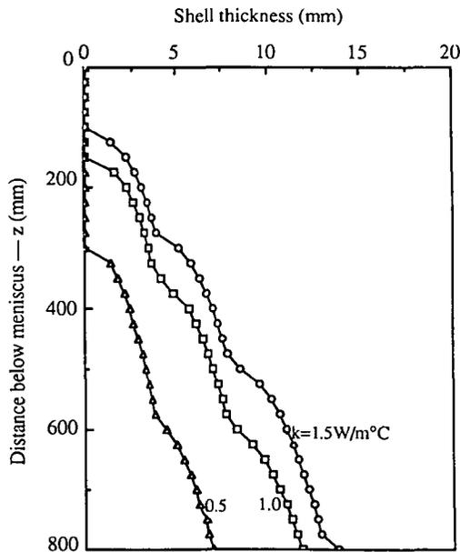
FIGURE 19. Effect of thermal conductivity  $k$  of the mould powder on the shell thickness on plane  $x=316$ mm.
