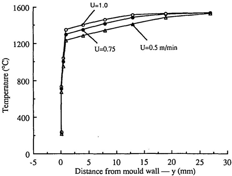
FIGURE 11. Effect of casting speed  $U$  of the steel on the temperature profile in line ( $x=316\text{mm}$ ,  $z=800\text{mm}$ ).
