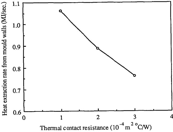
FIGURE 15. Effect of thermal contact resistance  $R$  on the overall heat extraction rate from the mould wall.
