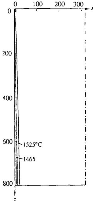
FIGURE 9. Temperature contours on the central vertical planes parallel to the broad face of the mould wall ( $y=201\text{mm}$ ).
