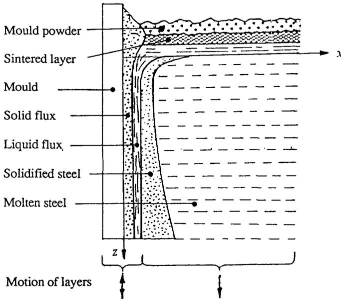
FIGURE 2. Various casting layers formed in mould.
