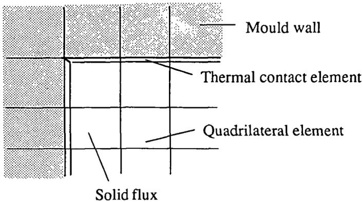
FIGURE 3. Discretized structure for the coupling of the mould wall and the solid flux regions.
