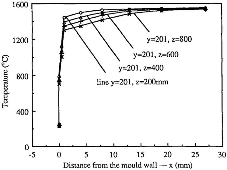
FIGURE 10. Distributions of temperature along various  $x$ -parallel lines.
