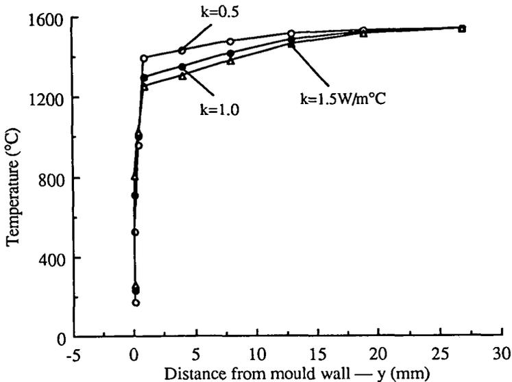
FIGURE 17. Effect of thermal conductivity  $k$  of the mould powder on the temperature profile in line ( $x=316\text{mm}$ ,  $z=800\text{mm}$ ).
