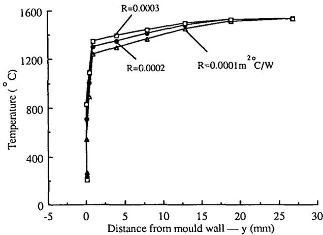
FIGURE 14. Effect of thermal contact resistance  $R$  on the temperature profile in line ( $x=316\text{mm}$ ,  $z=800\text{mm}$ ).
