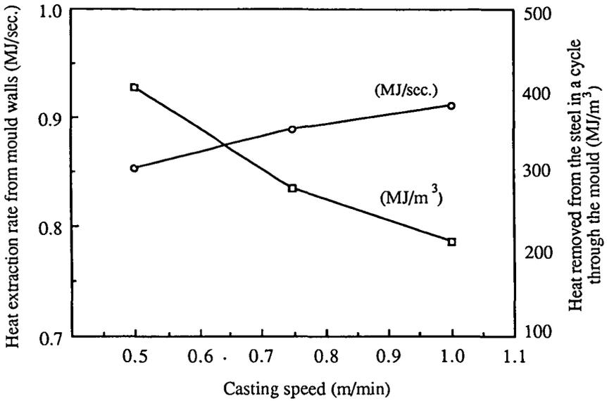
FIGURE 12. Effect of casting speed  $U$  of the steel on the overall heat extraction rate from the mould wall.
