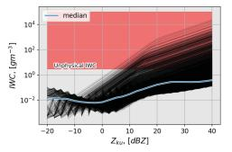
(b) Example of a partial dependency plot (Molnar, 2018) which shows how an AI model could product unphysical results when given unexpected inputs (Section 2.2.4). From (Chase et al., 2021). ©Molnar. Reproduced under the terms of the Creative Commons Attribution-NonCommercial-ShareAlike 4.0 International License (CC-BY-NC-SA 4.0).
