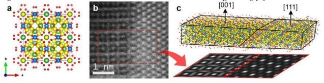
**Figure 1.** (a) Unit cell of cubic-LLZO lattice. (b) HAADF STEM image of LLZO containing a grain boundary. (c) Multislice STEM image simulation based on the atomistic model of a two-grain microstructure.
