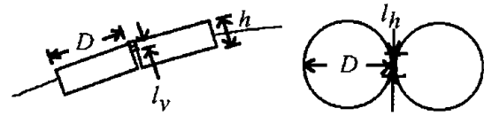
Fig. 3. Two floes frozen together on top of a wave field. The one on left is the side view and the one on right is the top view. The frozen area has a vertical dimension of l_\nu and horizontal dimension of l_h . Both floes can be composites of smaller floes formed at an earlier stage.
