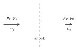
FIGURE 9. A shock front in its rest frame.
