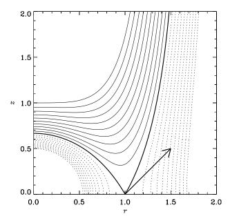
FIGURE 17. Contours of  $\Phi_{cg}$ , in units such that  $r_0 = 1$ . The downhill directions are indicated by dotted contours. If the inclination of the poloidal magnetic field to the vertical direction at the surface of the disc exceeds 30°, gas is accelerated along the field lines away from the disc.
