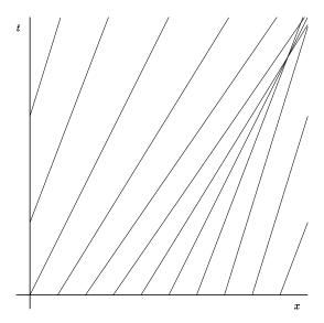
FIGURE 7. Formation of a shock from intersecting characteristics.
