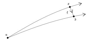
FIGURE 18. The Lagrangian displacement of a fluid element.
