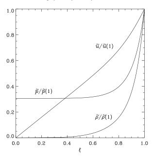
FIGURE 12. Sedov's solution for a spherical blast wave in the case  $\gamma = 5/3$ .
