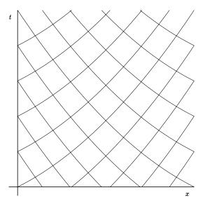
FIGURE 5. Characteristic curves in the space-time diagram.
