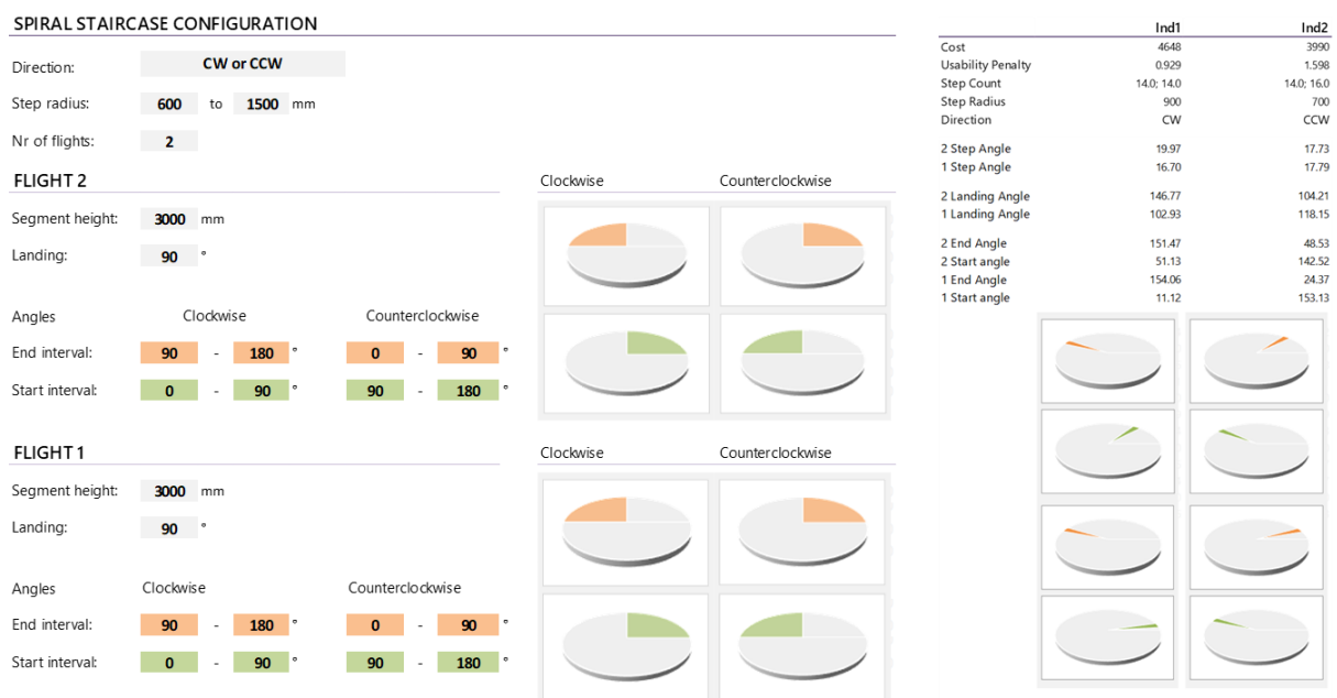
Figure 3. Proof-of-concept demonstrator for sales configurator with input (left) and result output (right) fields
