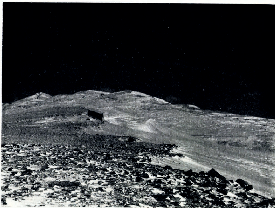
Fig. 4. Part of the long uniform snow field at Straight Creek on 15 December 1961. The fence was 2.4 m. tall and 55 m. long; it was lengthened to 90 m. during the summer of 1962. Control lines were located beyond the fence in an undisturbed part of the catchment
