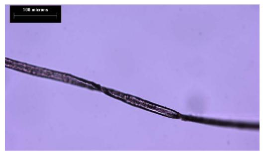
Figure 4 High-magnification image of a cotton fiber, crossed polars
