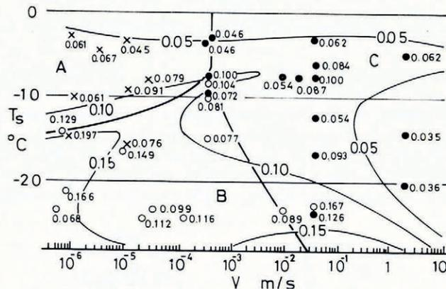
Fig. 4. Distribution of values of  $\mu_k$  plotted against temperatures and velocities (after Huzioka):
