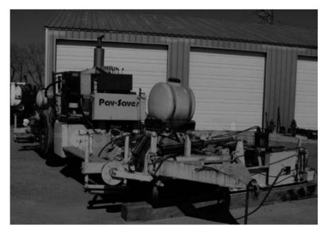
FIGURE 9.4 A Pav-Saver road-paving machine.
