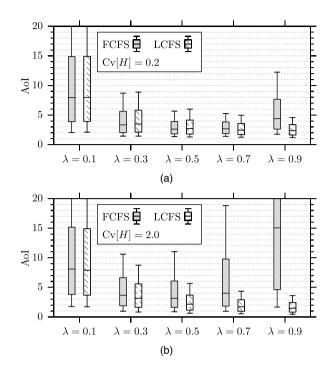
Figure 1.9 Comparison of the AoI distribution in FCFS and LCFS M/PH/1 queues.
