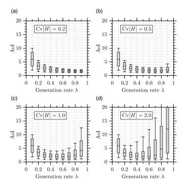
**Figure 1.8** Boxplots of the AoI distribution in the FCFS D/PH/1 queue. The whiskers represent 10 and 90 percentiles.
