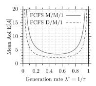
Figure 1.5 The mean AoI E[A] in the FCFS M/M/1 and D/M/1 queues.
