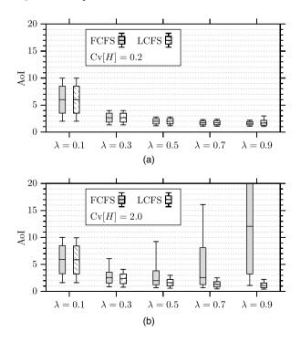
Figure 1.10 Comparison of the AoI distribution in FCFS and LCFS D/PH/1 queues.
