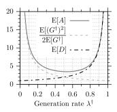
Figure 1.4 The mean AoI E[A] in the FCFS M/M/1 queue.
