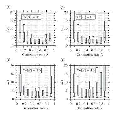
Figure 1.7 Boxplots of the AoI distribution in the FCFS M/PH/1 queue. The whiskers represent 10 and 90 percentiles.
