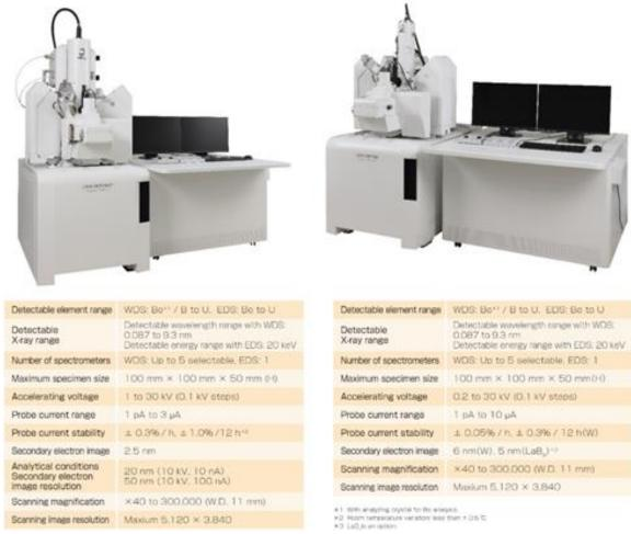
Figure 1. External appearance and principal specifications of the JXA-iHP200F and JXA-iSP100.
