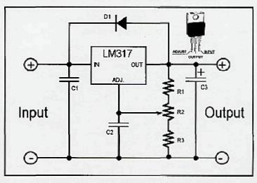
Circuit diagram for stable voltage source to replace mercury batteries
