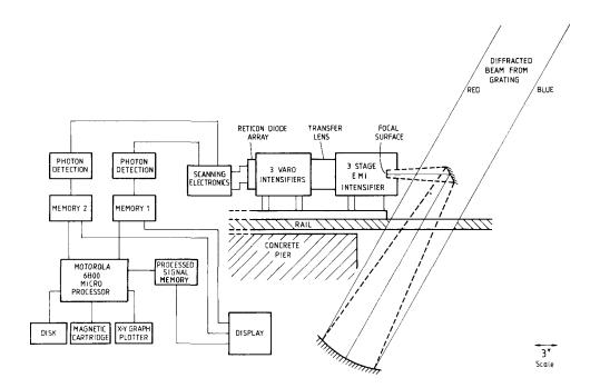
Figure 1. The 1 m camera in the RGO coudé spectrograph, showing the intensified Reticon system and associated processing electronics.
