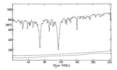
Figure 4. Sky spectrum in the region of the NaD lines shown as the mean of 10 pixels along the slit ( $\lambda$  increases to the left). The dotted line shows the mean background in these channels when no signal is present, whilst the dashed line is the mean of 10 strips from both sides of the spectrum on the exposed image, illustrating the amount of "smearing" observed.
