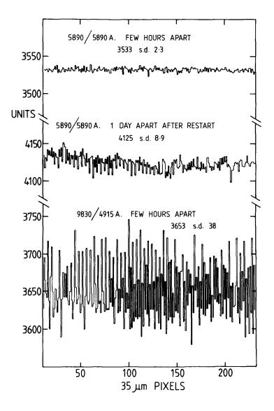
Figure 3. The top two records are flat field divisions at 5890A, where one unit represents approximately 170 photoelectrons. The bottom record shows division of two flat fields in widely separated spectral regions and demonstrates the difference in pixel-to-pixel variations at these wavelengths.
