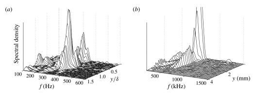
FIGURE 1. Power spectra at different heights above the cone surface for (a) low and (b) high-enthalpy conditions (from Laurence et al. (2016), figures 12 and 23).
