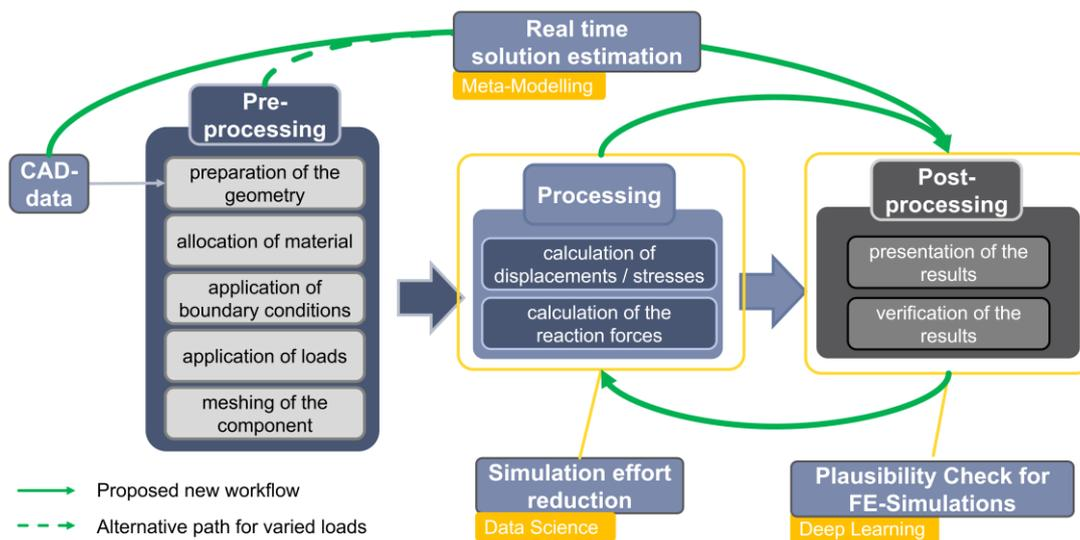
**Figure 3. Adapted process chain to perform an initial Design-Check**
