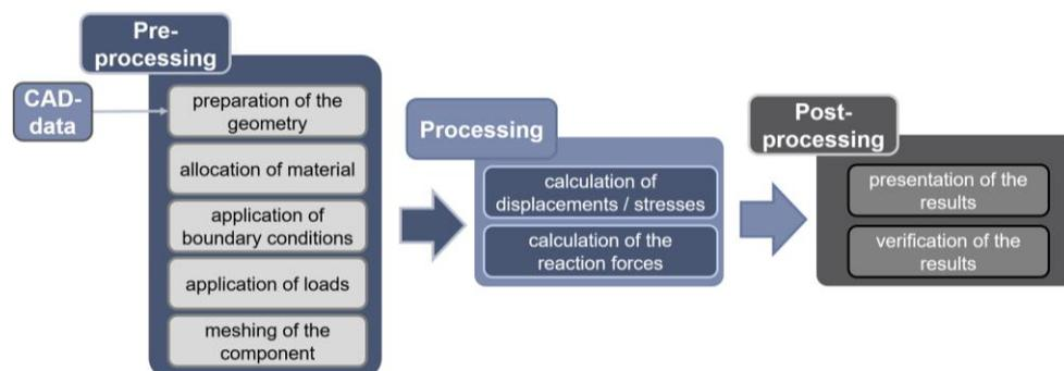
Figure 1. Simplified FE analysis process according to Vajna et al. (2018).
