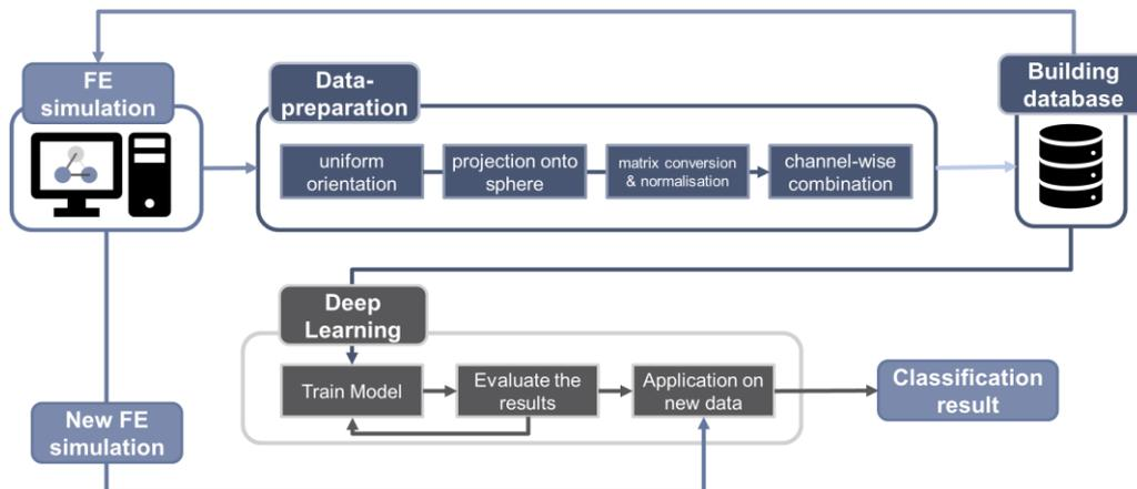
**Figure 7. Overview of the plausibility check procedure for FE-simulations**
