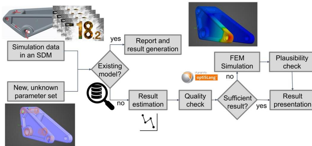
**Figure 4. Concept for initial design-checks**
