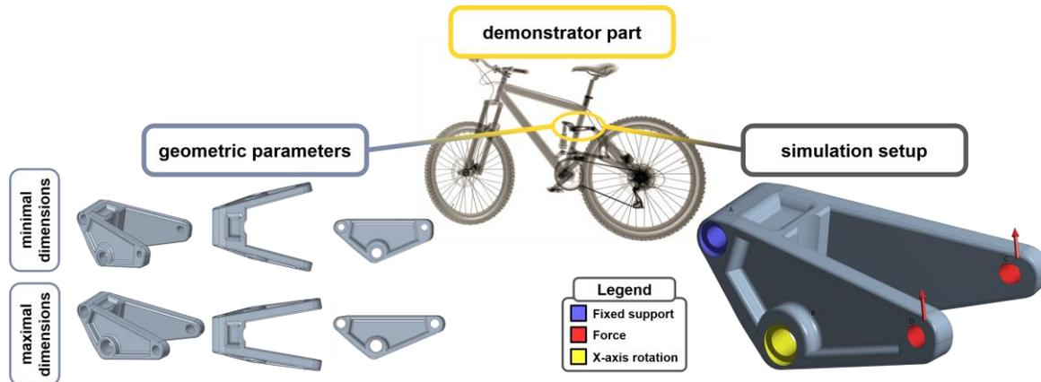
**Figure 5. Overview of the mountain bike rocker including its geometric parameter and the layout of the FE-simulation.**
