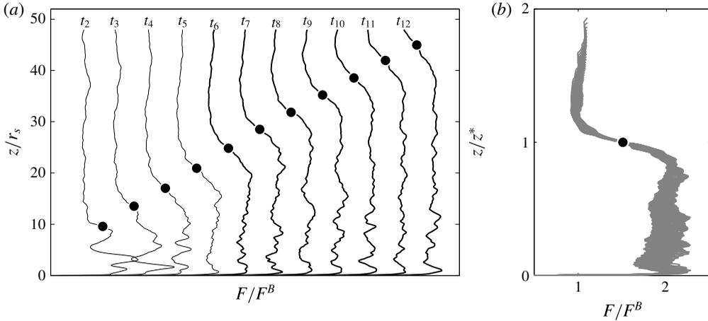
FIGURE 5. (a) Normalised buoyancy flux at the times  $t_n \approx 1.95\tau_s n$ . The black circle denotes  $z^*(t)$ , which corresponds to the location of the wave. Profiles  $t_2, \dots, t_5$  appear to be influenced by near-field effects and are therefore excluded from the plot in (b), which illustrates the self-similarity of the normalised buoyancy flux.
