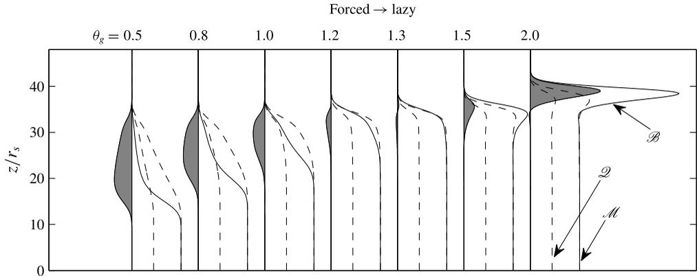
FIGURE 11. Wave structure for different values of  $\theta_g$ . The dashed lines are normalised integral quantities  $\mathcal{Q} \equiv Q/Q_0$ ,  $\mathcal{M} \equiv M/M_0$  and the solid line is  $\mathcal{B} \equiv B/B_0$ . The shaded region denotes the extent to which  $\Gamma(z, t)$  is different from unity. For  $\theta_g \approx 4/3$ ,  $\Gamma = 1$  and the wave is pure.
