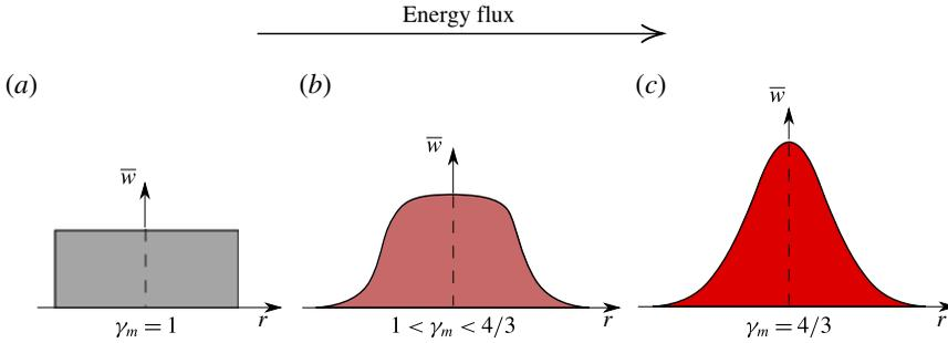
FIGURE 1. (Colour online) The mean dimensionless energy flux  $\gamma_m$  associated with different radial profiles of the longitudinal velocity. The top-hat profile (a) is a limiting case for which the dimensionless energy flux is minimal, while in the case of a Gaussian profile (c)  $\gamma_m = 4/3$ .
