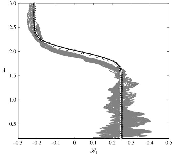
FIGURE 12. Predictions using a linearized, straight-sided, constant- $\Gamma$  model, for which  $\lambda^* = 2$ . The circles denote the prediction that is obtained by solving (6.22) numerically and the solid black line denotes the solution for  $Pe \gg 1$ . The grey lines correspond to observed values of the normalised buoyancy integral from the DNS at times in the interval  $[t_6, t_{12}]$  (cf. figure 5).
