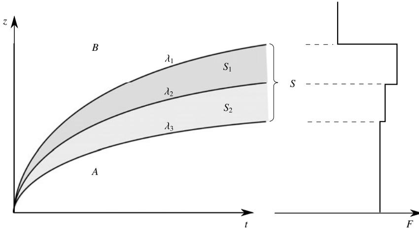
FIGURE 8. The three distinct characteristic curves and associated eigenvalues  $\lambda_1$ ,  $\lambda_2$  and  $\lambda_3$  in a generalised formulation of the unsteady plume equations. Regions *A* and *B* denote points in  $(z, t)$  space upstream and downstream of a wave, while regions  $S_1$  and  $S_2$  denote regions of the wave. The depicted behaviour of  $F$  in the wave is for schematic purposes only.
