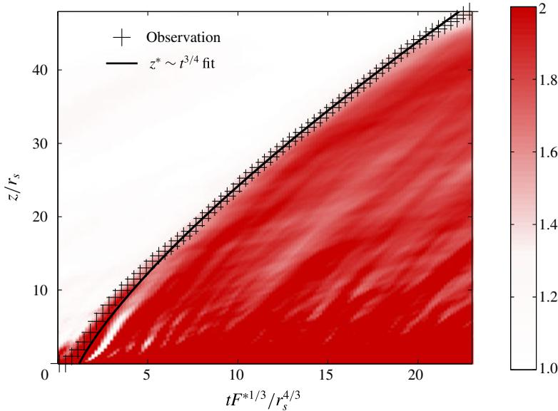
FIGURE 6. (Colour online) Dimensionless buoyancy  $b_m(z, t)/b_{m0}(z)$  in the plume, where  $b_{m0}$  is the steady-state buoyancy corresponding to simulation L with buoyancy flux  $F^B$ , in addition to points denoting the location of the travelling wave. The crosses correspond to the observed position of the front, while the line denotes a best fit to the front position, of the form  $z^* - z_v \propto (t - t_v)^{3/4}$ .
