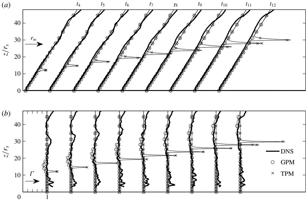
FIGURE 7. DNS data and model prediction of the plume radius  $r_m$  (a) and the flux-balance parameter  $\Gamma$  (b) at times  $t_n \approx 1.95\tau_s n$ . The thick solid line corresponds to the DNS data. GPM refers to the Gaussian plume model described in § 6 of this paper and TPM refers to the top-hat plume model described by Scase & Hewitt (2012). Note that the profiles in (b) are separated by a distance of 1 unit, as indicated by the scale in the bottom left corner.
