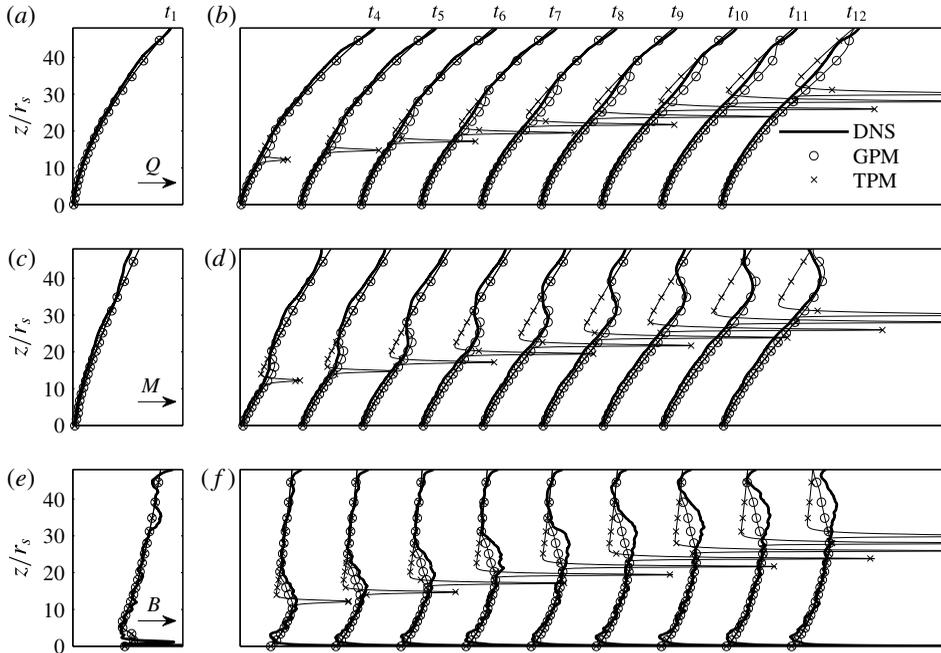
FIGURE 4. DNS data and model prediction of the volume flux  $Q$  (a,b); the momentum flux  $M$  (c,d); and the integral buoyancy  $B$  (e,f). (a,c,e) Display the initial conditions, while (b,d,f) display the data/predictions at times  $t_n \approx 1.95\tau_s n$ . The thick solid line corresponds to the DNS data. GPM refers to the Gaussian plume model described in § 6 of this paper, while TPM refers to the top-hat plume model described by Scase & Hewitt (2012).
