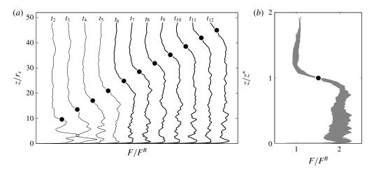
FIGURE 5. (a) Normalised buoyancy flux at the times  $t_n \approx 1.95\tau_s n$ . The black circle denotes  $z^*(t)$ , which corresponds to the location of the wave. Profiles  $t_2, \ldots, t_5$  appear to be influenced by near-field effects and are therefore excluded from the plot in (b), which illustrates the self-similarity of the normalised buoyancy flux.
