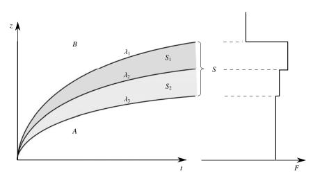
FIGURE 8. The three distinct characteristic curves and associated eigenvalues  $\lambda_1$ ,  $\lambda_2$  and  $\lambda_3$  in a generalised formulation of the unsteady plume equations. Regions A and B denote points in (z, t) space upstream and downstream of a wave, while regions  $S_1$  and  $S_2$  denote regions of the wave. The depicted behaviour of F in the wave is for schematic purposes only.
