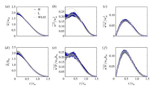
FIGURE 13. (Colour online) Normalised radial profiles of quantities in a steady-state plume. DNS data from simulations L and H are compared with the experimental data of Wang & Law (2002), which comprise a best fit to data obtained over the range  $62 < z/r_s < 110$ . The DNS data were obtained over the range  $20 < z/r_s < 40$ .
