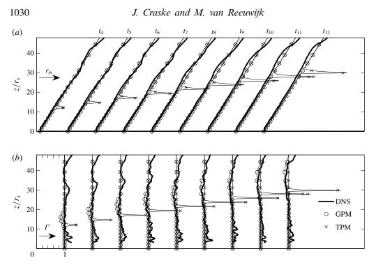
FIGURE 7. DNS data and model prediction of the plume radius  $r_m$  (*a*) and the flux-balance parameter  $\Gamma$  (*b*) at times  $t_n \approx 1.95\tau_s n$ . The thick solid line corresponds to the DNS data. GPM refers to the Gaussian plume model described in §6 of this paper and TPM refers to the top-hat plume model described by Scase & Hewitt (2012). Note that the profiles in (*b*) are separated by a distance of 1 unit, as indicated by the scale in the bottom left corner.
