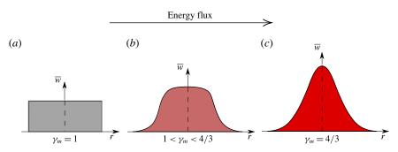
FIGURE 1. (Colour online) The mean dimensionless energy flux  $\gamma_m$  associated with different radial profiles of the longitudinal velocity. The top-hat profile (*a*) is a limiting case for which the dimensionless energy flux is minimal, while in the case of a Gaussian profile (*c*)  $\gamma_m = 4/3$ .
