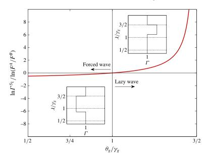
FIGURE 9. (Colour online) Wave structure in a straight-sided plume  $(\gamma_g/\beta_g = 4/3, \theta_m = 1)$ . The special case for which  $\Gamma = 1$  in the wave corresponds to  $\theta_g = \gamma_g$ . The variable  $\lambda$  is a scaled z coordinate, which is defined rigorously in (6.21).
