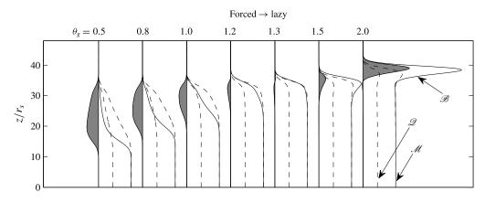
FIGURE 11. Wave structure for different values of  $\theta_g$ . The dashed lines are normalised integral quantities  $\mathcal{Q} \equiv Q/Q_0$ ,  $\mathcal{M} \equiv M/M_0$  and the solid line is  $\mathcal{B} \equiv B/B_0$ . The shaded region denotes the extent to which  $\Gamma(z, t)$  is different from unity. For  $\theta_g \approx 4/3$ ,  $\Gamma = 1$  and the wave is pure.
