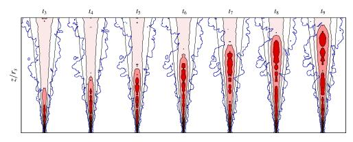
FIGURE 2. (Colour online) Isoregions of the ensemble and azimuthally averaged buoyancy (red) and threshold of the instantaneous enstrophy (blue) in an unsteady turbulent plume at times  $t_n \approx 1.95\tau_s n$ , n = 3, ..., 9, where  $\tau_s \equiv r_s^{4/3} (F_s^A)^{-1/3}$ . The buoyancy displayed in the figure has been non-dimensionalised using the local characteristic buoyancy scale  $b_{m0} \equiv B_0 M_0 / Q_0^2$  of a steady plume with buoyancy flux  $F^B$ .
