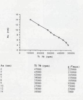
Table 2: First contrifugation: Beckman Centrifuge, Ti 70 rotor for 30 min at 4°C.
