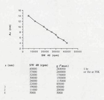
Table 3: Second centrifugation: Beckman Centrifuge, SW 40 rotor, 45 min 4° C,
