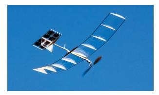
An ultralight perovskite solar panel integrated on the horizontal stabilizer of a model airplane's tail powers a DC motor with a propeller. The 64-cell solar panel generates 75 mW under ambient light conditions, enough to fly the airplane, which is 28cm long with a wingspan of 58 cm. Credit: Martin Kaltenbrunner/Johannes Kepler University Linz.
