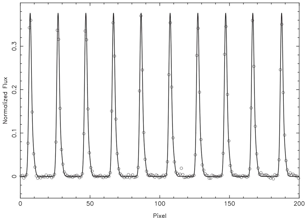
**Figure 2** Concatenation of emission lines from a group of fibres (hollow circles, corresponding to the  $\tilde{F}'$  function). Since there are no dead fibres in this group, ten emission lines were extracted and were used for the fit following the procedure described in the text. The best fit (the  $F'$  function) is shown as a thick line and faithfully represents the data. In particular, it reproduces the asymmetric, high-wavelength wing of each emission line.
