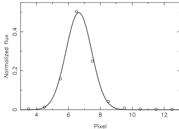
**Figure 7**  $8408.2096 \text{ \AA}$  CuAr emission line extracted from fibre 1 of a CCD2 calibration lamp observation (circles). The emission line is symmetric and can be fitted by a single Gaussian function of internal dispersion  $\sigma = 0.74$  (line).
