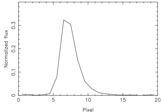
**Figure 1**  $5105.541\text{ \AA}$  Cu emission line extracted from fibre 1 of a CCD1 calibration lamp observation. The emission line shows an asymmetry towards higher wavelengths that accounts for  $\sim 30\%$  of the total signal.
