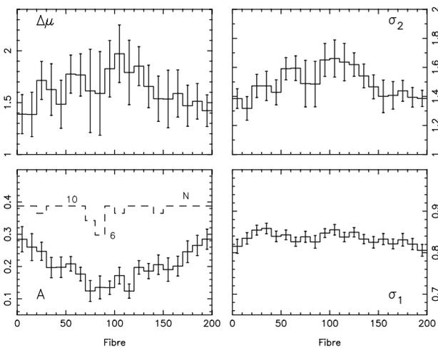
**Figure 3** Evolution of the four LSF-related parameters  $A$  (bottom-left panel),  $\sigma_1$  (bottom right),  $\sigma_2$  (top right), and  $\Delta\mu$  (top left) across CCD1. The three parameters representing the perturbation of the LSF ( $A$ ,  $\sigma_2$ , and  $\Delta\mu$ ) show substantial variations across the CCD. The number of fibres,  $N$ , used for the fit is plotted as a thin dashed histogram in the bottom-left panel.
