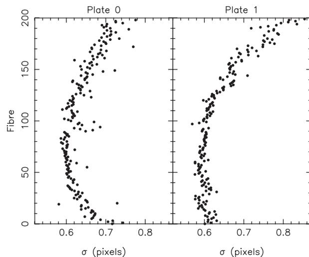
**Figure 8** Evolution of the internal dispersion,  $\sigma$ , of the LSF across CCD2 when fitted by a single Gaussian function as in Figure 7. Although the LSF remains symmetric across CCD2 (contrary to CCD1), its width varies substantially.
