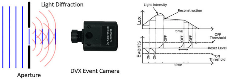
Figure 4. Event camera change in intensity.
