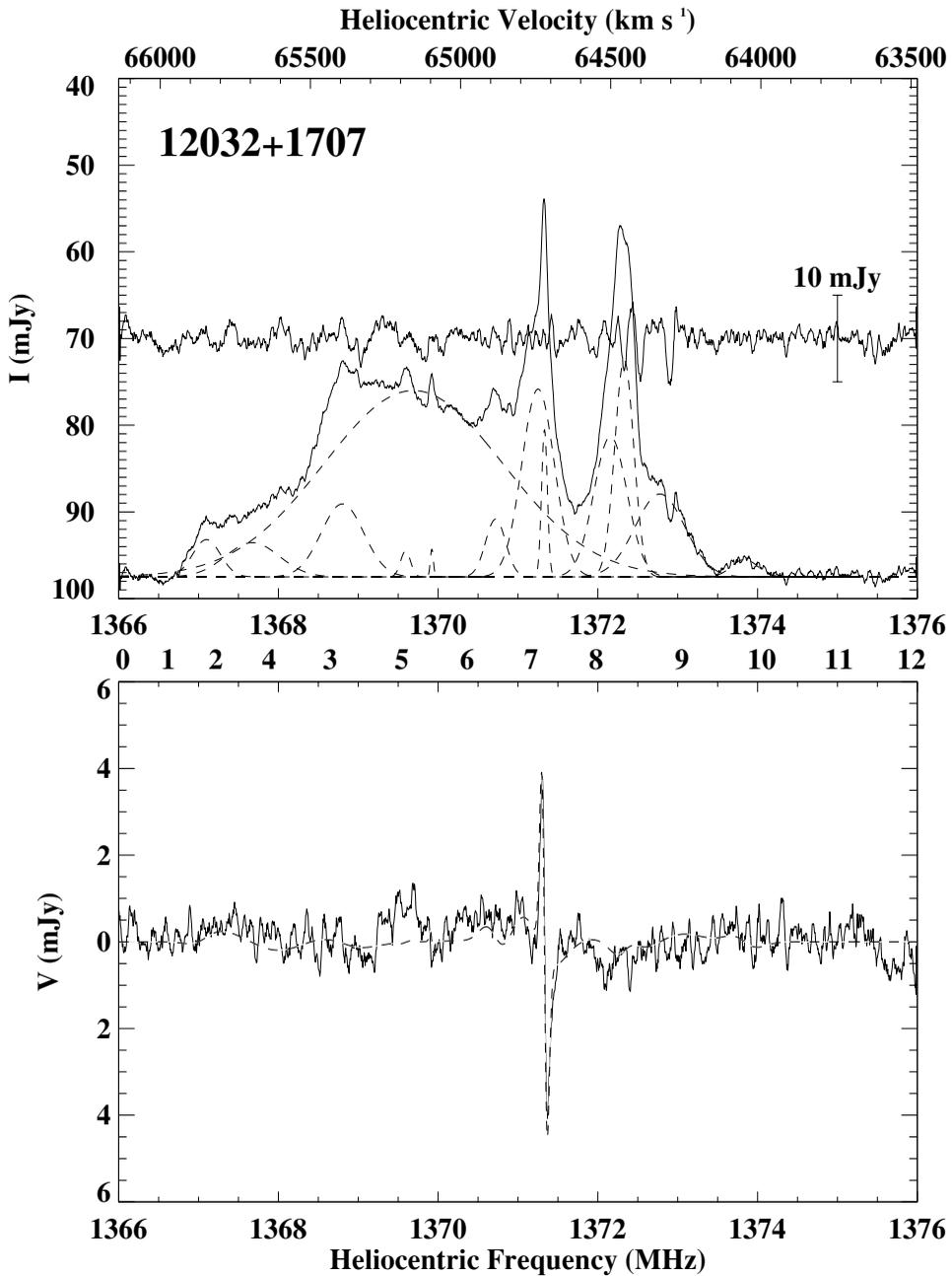
**Figure 1.** Stokes *I* spectrum (*top*) for IRAS F12032 + 1707. The residuals are plotted through the center of the Stokes *I* plot and are expanded by a factor of 2. The profile of each Gaussian component is plotted as a dashed line. The Stokes *V* (*bottom*) spectrum with its fit is plotted as a dashed line.
