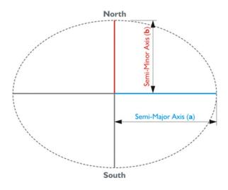
**Figure 2.** Meridian ellipse of an ellipsoid of revolution, where *a* and *b* are parameters in terms of which polar flattening  $(f = \frac{a-b}{a})$  is defined.
