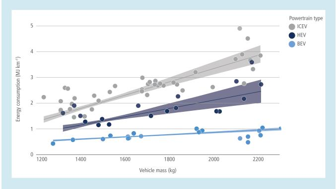
Box 10.3, Figure 1 | Illustration of energy consumption as a function of vehicle size (using mass as a proxy) and powertrain technology. FCVs omitted due to lacking data.
