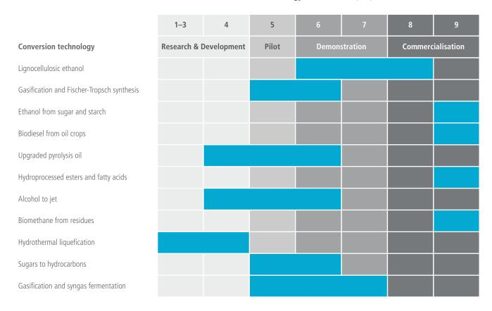
**Figure 10.3 | Commercialisation status of selected biofuels conversion technologies.** The blue boxes represent the current technology readiness level of each conversion technology. Source: based on Mawhood et al. (2016), Skeer et al. (2016), IEA (2017a), and Puricelli et al. (2021).
