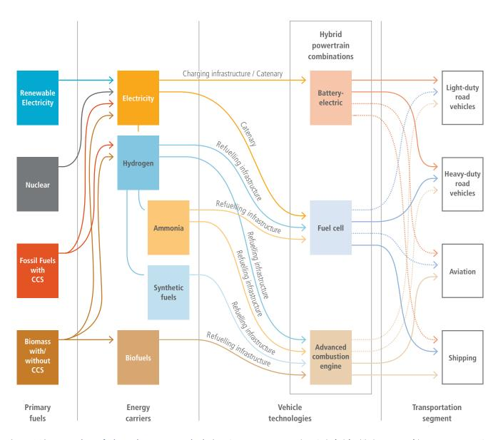
Figure 10.2 | Energy pathways for low-carbon transport technologies. Primary energy sources are shown in the far left, while the segments of the transport system are in the far right. Energy carriers and vehicle technologies are represented in the middle. Primary pathways are shown with solid lines, while dotted lines represent secondary pathways.
