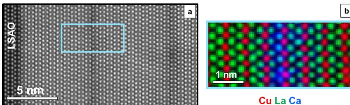
**Figure 2.** a) STEM-HAADF image of Ca-doped LCO superlattice showing a coherent interface and high structural quality. The image was taken along the [100] direction of the LSAO substrate. b) Atomically resolved EEL SI showing the elemental distribution of Cu (red), La (green), and Ca (blue).
