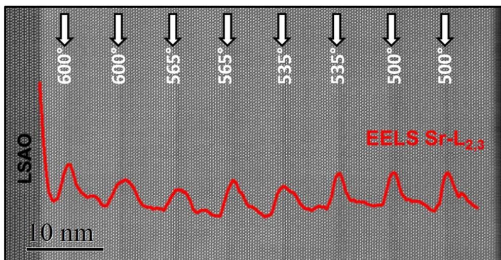
**Figure 1.** STEM-HAADF image of the Sr  $\delta$ -doped LCO superlattice showing the overview of the heterostructure with revealing the structural quality. The image was taken along the [100] direction of the LSAO substrate. The inset shows the integrated Sr-L<sub>2,3</sub> EELS line profile.
