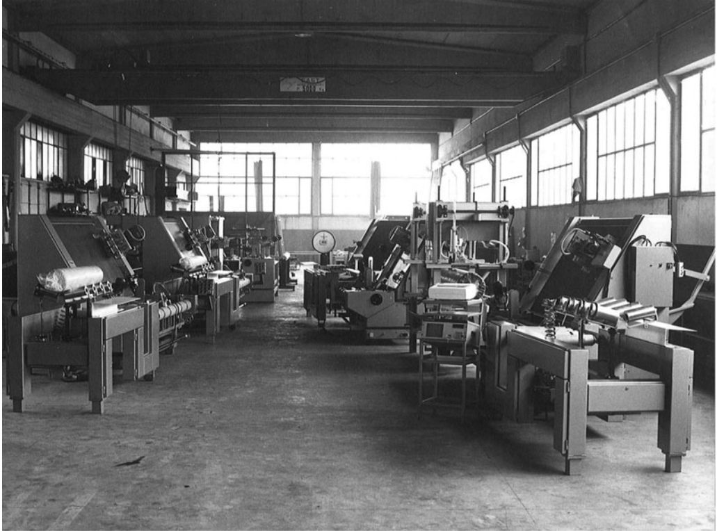
Figure 1. Early numerically controlled inspection and packing machines for textiles at the Testa factory in the Zanica industrial district north of Milan, 1969. Courtesy: Testa Group Archive.
