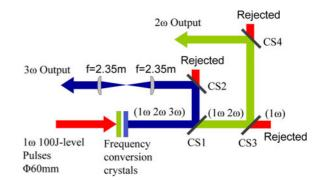
**Figure 11.** The frequency converter system layout. CS1–CS4, spectral mirrors with special coating layer.
