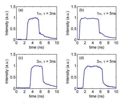
Figure 14. The  $1\omega$  and  $3\omega$  output 3 and 5 ns temporal pulses.
