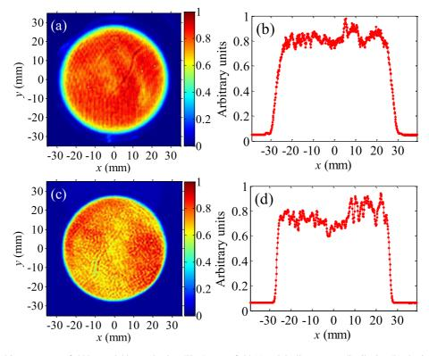
Figure 15. The 1 $\omega$  and 3 $\omega$  output near field by spatial beam shaping. The 1 $\omega$  near field (a) and the lineout gray distribution (b), the 3 $\omega$  near field (c) and the lineout gray distribution (d).
