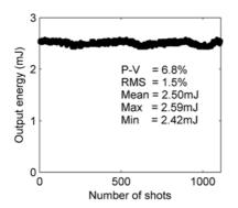
Figure 6. The energy stability of the preamplifier.
