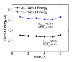
Figure 13. The output energy stability in six shots.
