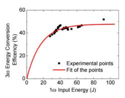
Figure 12. Conversion efficiency to third harmonic. The data are for a 5 ns input 1 $\omega$  pulse width and for a  $\Phi$ 58 mm beam.
