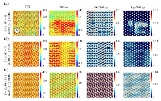
Figure 10. Regime (V): strand pulsations for the FENE-CR model with b = 1000. Each line corresponds to a set of dimensionless numbers with results presented for different time intervals. The first and second columns show the time-averaged fields of the trace of the conformation tensor and the corresponding r.m.s. variations, respectively. The third and fourth columns show the normalized time-averaged fields of the velocity and the corresponding r.m.s. variations, respectively.
