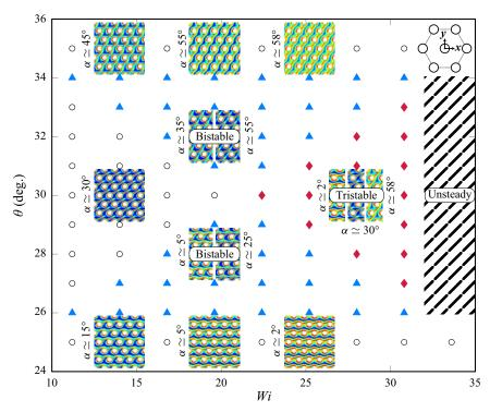
Figure 6. The  $(\theta, Wi)$  phase diagram with the different stability domains for the Oldroyd-B model with  $\beta = 1$ . Insets show the corresponding polymer stretching fields and the position of the strands;  $(\circ)$  indicates a single stable state,  $(\blacktriangle, blue)$  bistability and  $(\blacklozenge, red)$  tristability. Stripes indicate a transition towards unsteady flows.
