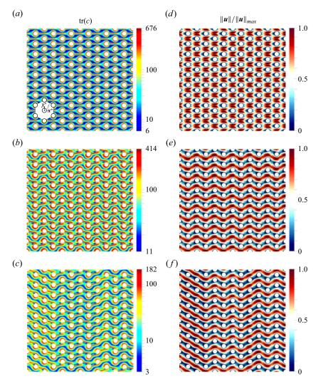
Figure 9. Examples of steady-state fields for tr(c) and the corresponding normalized amplitude of the velocity; (a)  $(\beta = 0.5, Wi = 42)$  corresponds to the trivial steady solution, (b)  $(\beta = 1, Wi = 53.2)$  to the regime (III) and (c)  $(\beta = 5, Wi = 19.6)$  to regime (IV).
