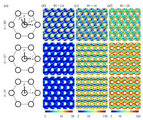
Figure 3. Steady viscoelastic flow through a hexagonal lattice of cylindrical obstacles. Fields of polymer stretching – the trace of the conformation tensor, tr(c) – for the Oldroyd-B model with a ratio of polymer to solvent viscosities  $\beta = 1$  and different values of the Weissenberg number Wi and angles  $\theta$  from the aligned configuration.
