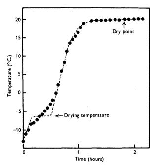
Fig. 9. Temperature curve recorded during the drying of 0.25 ml. of 'Mist. desiccans' by method 'B'. The black dots show the actual temperatures recorded. The broken line shows the assumed temperature curve, with a drying temperature at about  $-7^{\circ}$  C.
