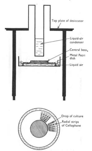
Fig. 7. Diagram of the apparatus used for drying with a liquid-air condenser for subsequent storage of the cultures. (Drying method 'A. 2'.)
