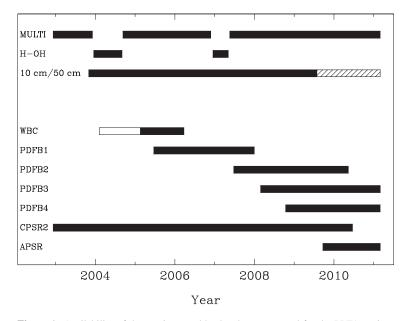
**Figure 1.** Availability of the receivers and backend systems used for the PPTA project. The hatched area on the 10-/50-cm bar indicates when the 50-cm band was retuned to operate in the 700–770 MHz (40 cm) band. The WBC bar is open when various instrumental problems affected the data quality. Significant intervals of overlap between operation of the various backend instruments allowed checks on instrument-dependent delays.
