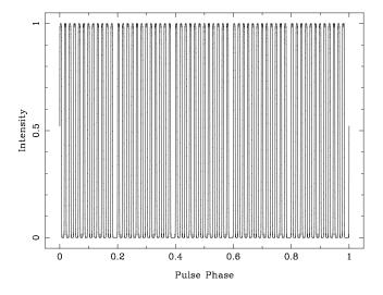
**Figure 5.** Template profile used for the measurement of instrumental delays for the PDFB3/4 configuration with 256 MHz bandwidth, 1024 channels, and 1024 profile bins. The rectangular input waveform has a leading edge at phase 0.0; the convolution for the finite channel bandwidth smears the edge transitions by a small amount.
