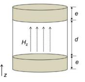
**Fig. 11.** Scheme of a fully enclosed cavity loaded with dielectric segements with height *e*. The AMC boundary conditions, for which the mode in the central region (considered empty) is  $TE_{o10}$ , have length  $e = e_a$  given in equation (7).
