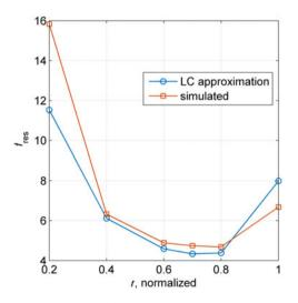
**Fig. 15.** Intrinsic resonance frequency associated to the loop-gap structure as function of the internal radius *r*. All dimensions are as the reported in Table 1, the normalization is according r = 16.8 mm. The outcome of equation (11) is compared to a result from full-wave eigen simulation performed via ANSYS HFSS. By applying PMC boundaries at both planes of the loop-gap cross-section, the numerically found frequency has the same physical meaning as the modeled in equation (11).
