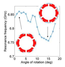
**Fig. 20.** Change of the resonance frequency corresponding to different rotation angles of the tuning electrodes (shown in blue) with respect to the loop gap (shown in red).
