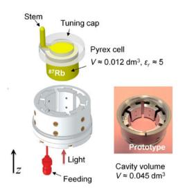
**Fig. 10.** Scheme of an atomic clock cavity based on a loop-gap structure [14]. Realizations that additionally include optical lens are also possible. A variety of dielectric materials can be used for the vapor cell. A high level of customization is required due to the different structures of the condensation stems that can be used in practice.
