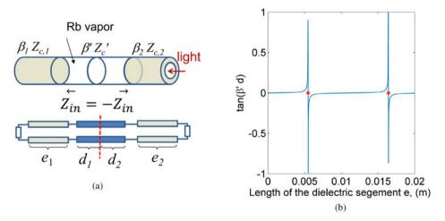
Fig. 13. Transmission line model and numerically obtained solution for the transcendental equation (9). The roots are indicated with red markers and correspond to the first two solutions found for the length *e* for which the dielectric segments appear as AMC boundary condition. The calculated result corresponds to the previously discussed cavity geometry – Fig. 12 and confirms the result obtained via equation (7).
