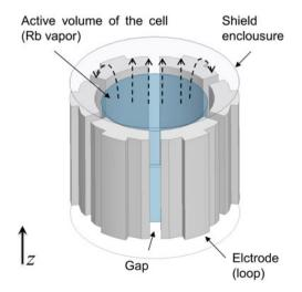
**Fig. 9.** Scheme of the basic structure of atomic clock cavity. The loop-gap structure is based on six electrodes. Two empty cylindrical extensions are situated on both sides of the loop-gap region. The magnetic field lines are represented by the dashed arrows. The components required for the clock operation are omitted (e.g. vapor cell, apertures required for the pumping light, optical lenses, feeding, tunning mechanism).
