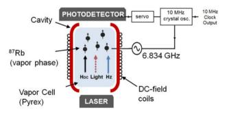
**Fig. 2.** The rubidium atoms in vapor phase are enclosed in a dielectric cell (Pyrex) situated inside the microwave cavity. Two apertures allow the laser light to penetrate, interact with the atoms, and get detected by the photo-detector. The *C*-field required for the Zeeman splitting is created by the coils surrounding the cavity oriented in the *z*-direction.
