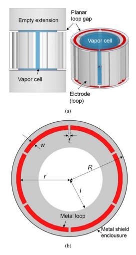
Fig. 16. Loop-gap cavity with AMC boundaries based on planar structures.
