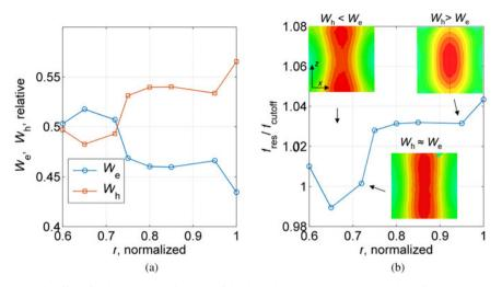
**Fig. 17.** The plots show what is the effect of scaling the internal radius *r* of the planar loop gap. For normalized radius of  $\approx$  0.72, the mode in the central region is TE<sub>010</sub> and the cavity resonates at the cutoff (of the central region). All dimensions are as reported in Table 1. The height of the extensions is 14 mm, and the distance between the planar loop gap and the central region is 1 mm.
