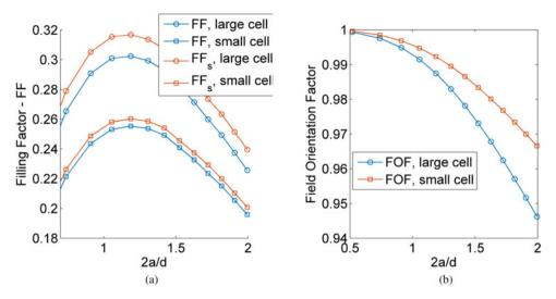
**Fig. 6.** Figures of merit for the  $TE_{011}$  cylindrical cavity as function of the cavity dimensions (radius – *a*, height – *d*). Two cylindrical vapor cells are considered: "small", b = 10 mm, l = 20 mm; large, b = 11 mm, l = 23 mm (Fig. 3).
