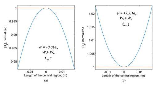
**Fig. 14.** The plots show the effect of the dielectric length on the  $H_z$  distribution in the homogeneous region of the cavity. The result is calculated for the central axis of a TE<sub>010</sub> cavity with radius of 26.7 mm and length of 36.6 mm. Dielectric with  $\epsilon_r = 5$  is considered. The field profiles are normalized with respect to the center of the cavity, and the constant field distribution corresponding to the ideal AMC case is shown in red.
