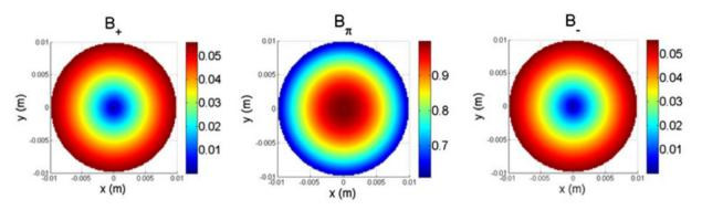
Fig. 4. Simulated 2D field profiles corresponding to the driving fields that interact with the atoms inside the vapor cell. The field amplitudes are averaged along the direction of the laser light – z and are shown normalized to the maximum found in the center for in case of the TE<sub>011</sub> mode. Each component is color-coded separately.
