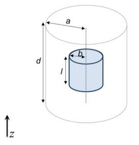
**Fig. 3.** Scheme of cylindrical cavity loaded with vapor cell (shown in blue). The position of the cell is chosen such that large fraction of the atoms inside the cell can interact with the  $B_z$  component – TE<sub>011</sub> mode is assumed.
