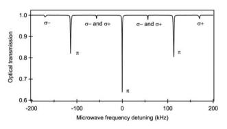
**Fig. 5.** Zeeman-split spectrum of the atomic microwave transition, recorded in continuous-wave double-resonance mode. The central line around zero frequency detuning corresponds to the required clock transition for which the cavity needs to be designed to maximize.
