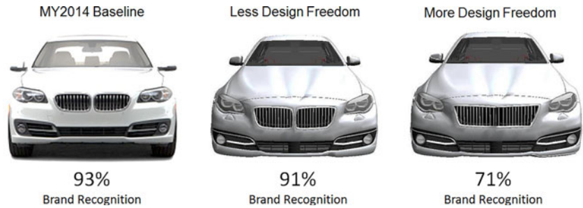
Figure 12. Example application to industry of the approach and results of this study. Three representations are given corresponding to the MY2014 Baseline BMW 5 Series, the morphed BMW 5 Series with the least design freedom from the baseline, and the morphed BMW 5 Series with the most design freedom from the baseline according to the data. Note that the MY2014 baseline is a 2D image, while the two morphed vehicles are images of the 3D morphing model.
