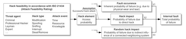
Figure 7. Calculation of probability of failure
