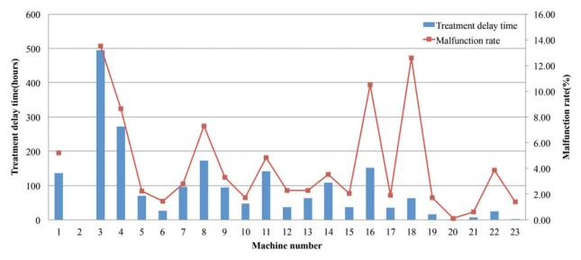
Figure 5. Treatment delay time and malfunction rate of TOMO units over 1 year.
