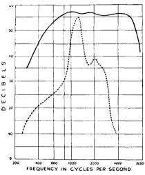
The poor results given by the ordinary electrical hearing aid consisting of a microphone, earphone, and dry battery are due to noise in the carbon granule microphone, and to frequency and amplitude distortion.
