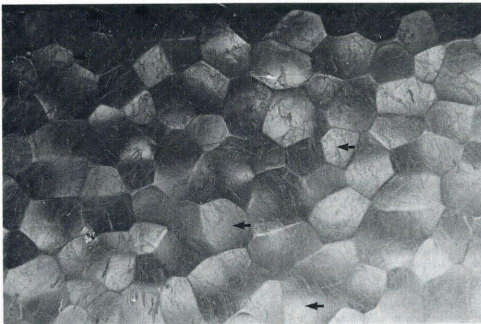
*Fig. 2. Photograph of the upper surface of the ice using side lighting showing the regular hexagonal pattern of the cavities. The fine hair-like structures show internal defects in the ice and thermally etched grain boundaries on the surface (arrows).*
