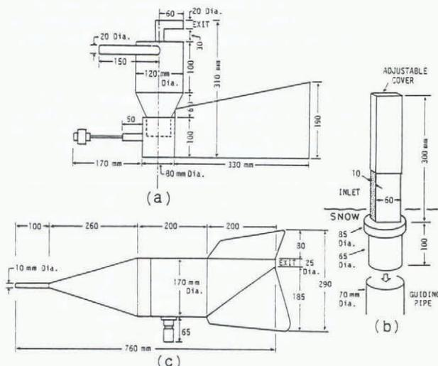
Fig.1. Snow drift collectors: (a) cyclone type with vanes, (b) slit type, and (c) rocket type.
