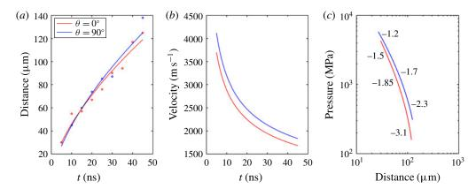
FIGURE 11. (Colour online) (a) The distance between plasma and shock front versus the elapsed time. (b) The velocity of the shock wave versus the elapsed time. (c) The pressure of the shock wave versus the distance between the plasma and shock front. The inserted numbers indicate the local slope of the corresponding curve.
