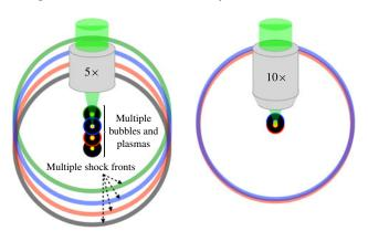
FIGURE 6. (Colour online) Schematic of a multiple structure model for a laser-induced underwater shock wave. Multiple plasmas emit multiple bubbles and spherical shock waves. The shock pressure at a certain point is the sum of the spherical shock pressures that reach the same point.
