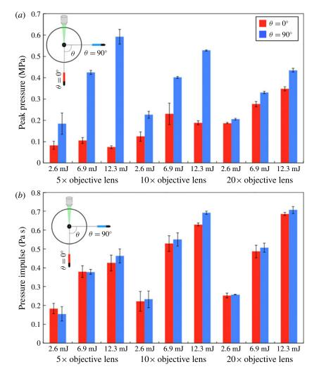
FIGURE 5. (Colour online) (a) Peak pressure of a laser-induced underwater shock wave measured at  $\theta=0^\circ$  and  $\theta=90^\circ$  for all the experimental conditions. Each presented value is a mean of three measurements and the error bars show the standard deviations. (b) Pressure impulse of a laser-induced shock wave measured at  $\theta=0^\circ$  and  $\theta=90^\circ$  for all the experimental conditions.
