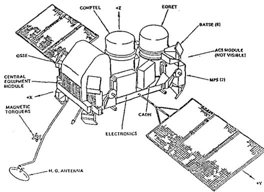
Figure 1. The Gamma Ray Observatory
