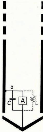
Fig. 1. Diagrammatic sketch of proposed method of measuring permittivity and hence temperature of ice using a thermal boring head
