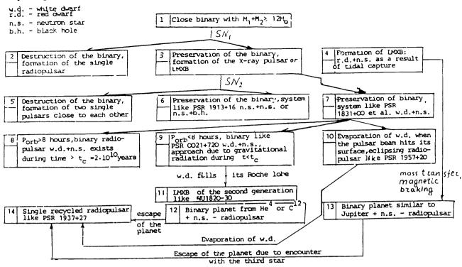
Figure 1 Scheme of evolutionary formation of recycled pulsars.
