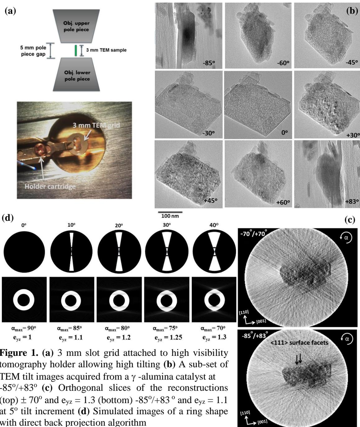
**Figure 1.** (a) 3 mm slot grid attached to high visibility tomography holder allowing high tilting (b) A sub-set of TEM tilt images acquired from a  $\gamma$ -alumina catalyst at  $-85^\circ/+83^\circ$  (c) Orthogonal slices of the reconstructions (top)  $\pm 70^\circ$  and  $e_{yz} = 1.3$  (bottom)  $-85^\circ/+83^\circ$  and  $e_{yz} = 1.1$  at  $5^\circ$  tilt increment (d) Simulated images of a ring shape with direct back projection algorithm
