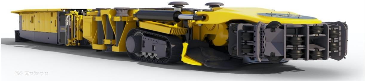
Figure 1. An example of a mobile miner. The cutter wheel can be seen to the right in the figure. Image reproduced from [Epiroc, 2021](#) with permission, © Epiroc.
