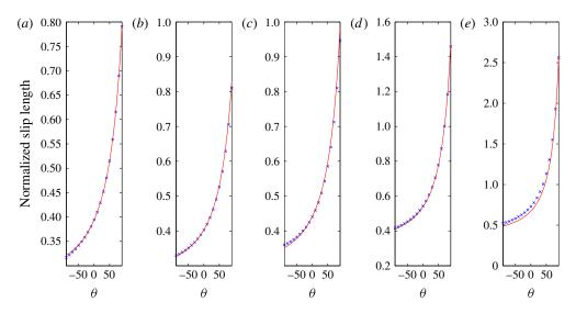
FIGURE 3. Normalized slip length, now based on the approximation  $\lambda_2$  in (4.13), as a function of  $\theta$  for c/l = 0.1 (a), 0.25 (b), 0.5 (c), 0.75 (d) and 0.9 (e). Crosses show numerical data from Teo & Khoo (2010).
