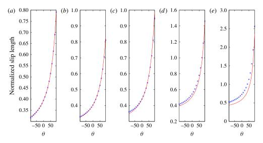
FIGURE 2. Normalized slip length (3.7) as a function of protrusion angle  $\theta$  for c/l = 0.1 (a), 0.25 (b), 0.5 (c), 0.75 (d) and 0.9 (e). Crosses show numerical data from Teo & Khoo (2010).
