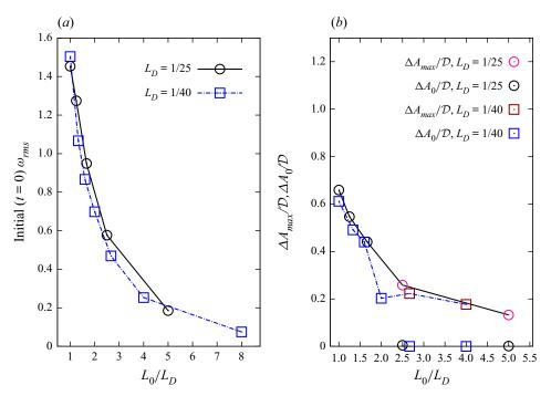
Figure 11. Initial shear, i.e. r.m.s. vorticity as a function of  $L_0/L_D(a)$  and largest step size (jump in area)  $\Delta A_{max}$  (or  $\Delta A_0$  in the case that  $q \approx 0$  on the largest mixed area) normalized by the domain area  $\mathcal{D}$  as a function of  $L_0/L_D(b)$  for simulations with  $L_D = 1/25$  (open circles) and  $L_D = 1/40$  (open squares).
