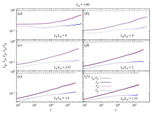
Figure 3. Time evolution of centroid length scales  $\ell_E$  of the total energy (solid black line),  $\ell_P$  of the potential energy (dashed magenta line) and  $\ell_K$  of the kinetic energy (dotted blue line) for simulations with  $L_D = 1/40$  and  $L_0/L_D = 8$  (*a*),  $L_0/L_D = 4$  (*b*),  $L_0/L_D = 2.67$  (*c*),  $L_0/L_D = 2$  (*d*),  $L_0/L_D = 1.6$  (*e*) and  $L_0/L_D = 1.33$  (*f*). The ratio  $\ell_E/\ell_P$  (black dash-dot line) is also shown.
