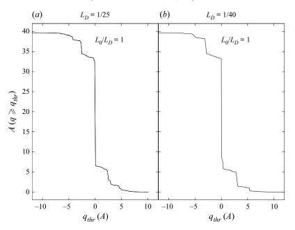
Figure 8. Potential vorticity staircases for simulations with  $L_D = 1/25$ ,  $L_0/L_D = 1$  (*a*, *t* = 200 000) and  $L_D = 1/40$ ,  $L_0/L_D = 1$  (*b*, *t* = 604 500). The structures are the same, suggesting the staircase structure depends only on the ratio  $L_0/L_D$ .
