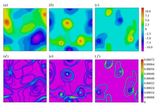
Figure 4. Potential vorticity (a-c) and kinetic energy (d-f) for simulations with  $L_D = 1/25$  and  $L_0/L_D = 5$  (*a*,*d*),  $L_0/L_D = 1.67$  (*b*,*e*) and  $L_0/L_D = 1$  (*c*,*f*), all at  $t = 200\,000$ . The domain length  $L = 2\pi$  is 25 deformation wavelengths  $2\pi L_D$ .
