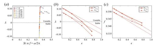
Figure 20. (a) Eigenvalues of the uncontrolled ( $\epsilon = 0$ ) and controlled ( $\epsilon \in [0; 0.75]$ ) flow with a force modelled by (3.1) for increasing  $\epsilon$  and located at the station ( $x_c^*$ ,  $y_c^*$ ). The sweep angle is  $\Lambda = 0^\circ$ , the angle of attack  $\alpha = 20^\circ$  and the Reynolds number is Re = 220. (b) Growth rate and (c) frequency as a function of the amplitude  $\epsilon$  for the most unstable global modes depicted in panel (a).
