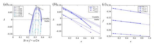
Figure 19. (a) Eigenvalues of the uncontrolled ( $\epsilon = 0$ ) and controlled ( $\epsilon \in [0; 0.75]$ ) flow with a force modelled by (3.1) for increasing  $\epsilon$  and located at the station ( $x_c^*$ ,  $y_c^*$ ). The sweep angle is  $\Lambda = 25^\circ$ , the angle of attack  $\alpha = 20^\circ$  and the Reynolds number is Re = 220. (b) Growth rate and (c) frequency as functions of the amplitude  $\epsilon$  for the most unstable global modes depicted in panel (a).
