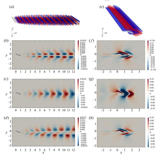
Figure 14. Direct and adjoint leading global mode for  $\Lambda=25^{\circ}$ ,  $\alpha=20^{\circ}$  and Re=190: contours of the real part of the streamwise velocity of (a) the direct global mode and (e) the adjoint one. (b-d) Slices in the spanwise plane z=0 ( $L_z=8$ ) of (b) streamwise, (c) cross-stream and (d) spanwise velocity components for the direct mode, and (f-h) the same for the adjoint one, respectively.
