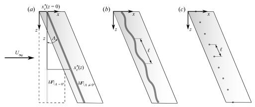
Figure 21. Sketch of the geometry for the application of the steady force (a) homogeneously along the swept wing, (b) modulated along the span and (c) as pointwise spheres.
