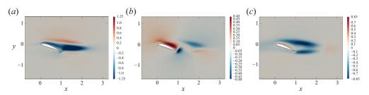
Figure 15. Spatial distribution in the plane z=0 of the growth-rate sensitivity to a steady force of the leading eigenvalue for  $\Lambda=25^{\circ}$ ,  $\alpha=20^{\circ}$  and Re=190: (a) streamwise, (b) cross-stream and (c) spanwise components of  $\nabla_F \lambda$ .
