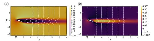
Figure 4. Base flow of the periodic  $25^{\circ}$  swept wing: spatial distribution of (a) the streamwise component U and (b) the spanwise component W of the velocity field in the spanwise plane z=0 for  $\alpha=20^{\circ}$  and Re=400. The white solid lines represent the corresponding velocity profiles at the streamwise locations x/c=1.25, 2, 2.75, 3.5, 4.25 and 5, while the dashed ones refer to the unswept wing at the same flow conditions.
