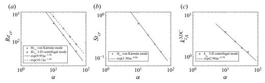
Figure 6. Marginal curves in log-log plots for the flow around a periodic unswept wing: (a) the emergence threshold of the two-dimensional von Kármán mode together with that of the three-dimensional centrifugal mode in the  $\alpha$ -Re plane; (b) the critical Strouhal number of the von Kármán mode; and (c) the spanwise wavenumber  $k_{z_A}$  of the leading three-dimensional centrifugal mode as a function of the angle of attack.
