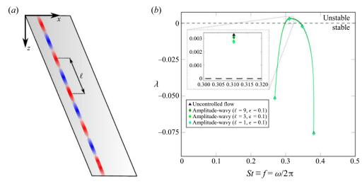
Figure 27. (a) Sketch of the geometry for the application of the amplitude-wavy steady force and (b) eigenvalues of the uncontrolled ( $\epsilon = 0$ ) and controlled flow with the amplitude-wavy forcing located at the station ( $x_c^*$ ,  $y_c^*$ ). The sweep angle is  $\Lambda = 25^\circ$ , the angle of attack  $\alpha = 20^\circ$  and the Reynolds number is close to the bifurcation, i.e. Re = 190. The spanwise extent is  $L_z = 8$ . See also table 7.
