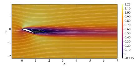
Figure 3. Base flow of the periodic unswept wing: spatial distribution of the streamwise velocity U in the spanwise plane z = 0 ( $L_z = 8$ ) for  $\alpha = 20^{\circ}$  and Re = 180. The white solid lines represent the streamlines and the single blue one is the locus of the points where the streamwise velocity of the base flow is zero, i.e. the recirculation bubble region.
