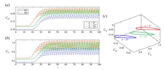
Figure 2. Time histories of (a) the drag and (b) the lift coefficients obtained from the two sets of meshes, M1 and M2, at  $\alpha=20^{\circ}$  and Re=400 and for three sweep angles,  $\Lambda=0^{\circ}$ ,  $12^{\circ}$ ,  $25^{\circ}$ . (c) Flow attractor via representation of aerodynamic coefficients from the grid M2 once the two-dimensional von Kármán mode is established for  $\alpha=20^{\circ}$  and Re=400.
