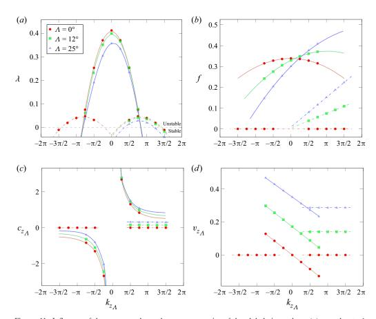
Figure 11. Influence of the sweep angle on the wave properties of the global eigenvalues: (a) growth rate  $\lambda$ , (b) frequency f, (c) phase velocity  $c_{z_A}$  and (d) group velocity  $v_{z_A}$  as functions of the spanwise wavenumber  $k_{z_A}$  at  $\alpha=20^\circ$  and Re=400 for  $\Lambda=0^\circ$ ,  $12^\circ$ ,  $25^\circ$ .
