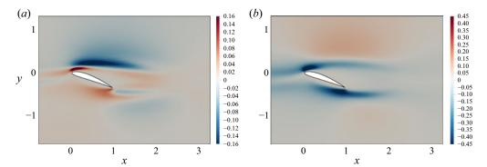
Figure 17. Variations of (a) the growth rate  $\delta \lambda / \epsilon$  and (b) the frequency  $\delta \omega / \epsilon$  in the plane z = 0 as a function of the location of the steady force modelled by (3.1). The results are given for  $\Lambda = 25^{\circ}$ ,  $\alpha = 20^{\circ}$  and Re = 190.
