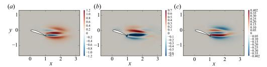
Figure 26. Spatial distribution in the plane z=0 of the frequency sensitivity to a base-flow modification of the leading eigenvalue for  $\Lambda=25^\circ$ ,  $\alpha=20^\circ$  and Re=190: (a) streamwise, (b) cross-stream and (c) spanwise components of  $\nabla_{U}\omega$ .
