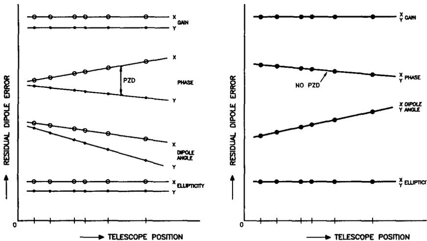
Fig. 1. Illustration of the nature of the absolute errors that cannot be determined with redundancy calibration, for the case of parallel dipoles (left) and crossed dipoles (right). For the latter, a single combined solution exists for both X- and Y-dipoles, eliminating the "offset-difference" problems.
