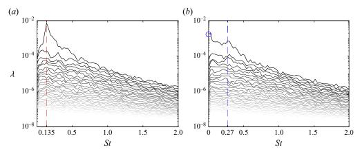
Figure 15. SPOD spectra at x/D = 10, for (a) m = 1, and (b) m = 2. Dashed red and blue lines in (a) and (b) correspond to St = 0.135 and St = 0.27, respectively.
