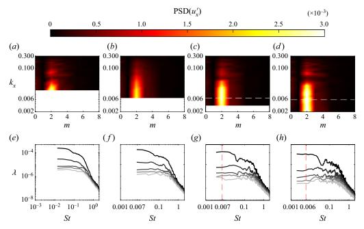
Figure 19. Effect of  $n_{fft}$  and tapers on (a-d) the PSD at r/D = 2, x/D = 40, and (e-h) SPOD at x/D = 40, for:  $(a,e) n_{fft} = 1024$ ,  $N_{win} = 10$ ;  $(b,f) n_{fft} = 2048$ ,  $N_{win} = 10$ ;  $(c,g) n_{fft} = 4096$ ,  $N_{win} = 10$ ;  $(d,h) n_{fft} = 7132$ ,  $N_{win} = 10$ . The white and red lines correspond to the peak in PSD and SPOD spectra. The PSD and SPOD spectra are plotted for St > 0.
