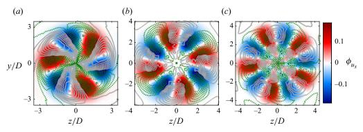
Figure 14. Leading SPOD mode at x/D = 40 and  $St \to 0$  for higher azimuthal wavenumbers, for (a) m = 3, (b) m = 4, and (c) m = 5. The false colours represent  $\operatorname{Re}[\phi_{u_x}^{(1)}(St \to 0)]$ , and the grey lines and green dotted lines correspond to the positive and negative values of streamwise vorticity  $\operatorname{Re}[\phi_{\omega_x}^{(1)}(St \to 0)]$ .
