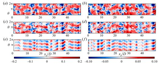
Figure 4. Streamwise velocity fluctuations  $u'_x$  on an  $x_t/D-\theta$  plane at  $r/D \approx 0.8$ , for  $(a,c,e) x_0/D = 10$ , and  $(b,d,f) x_0/D = 20$ . Plots (a,b) include all azimuthal components; (c,d) exclude m = 1; and (e,f) include solely m = 2.
