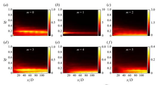
Figure 8. Percentage of energy contained in the leading SPOD modes  $\lambda^{(1)}$  as a function of frequency *St* and streamwise location x/D at different azimuthal wavenumbers: (a) m = 0, (b) m = 1, (c) m = 2, (d) m = 3, (e) m = 4, and (f) m = 5. The leading SPOD eigenvalue  $\lambda^{(1)}(St, x/D)$  is normalized with the total TKE  $E_k^T(x/D)$  at the corresponding streamwise location, to calculate the percentage contribution.
