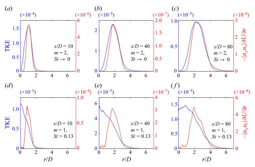
Figure 11. TKE and production due to shear at different downstream locations for the flow fields reconstructed from (a-c) the streaky-structures mode, and (d-f) VS mode. Plot (a,d) correspond to x/D = 10, (b,e) to x/D = 40, and (c,f) to x/D = 80. Flow reconstruction uses the leading five SPOD modes.
