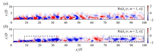
Figure 1. Azimuthally decomposed instantaneous fields of the streamwise velocity  $(u_x)$  for (a) m = 1 and (b) m = 2 azimuthal modes. Rectangular boxes in (b) show large-scale streaks in the m = 2 field.
