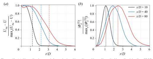
Figure 13. (a) Normalized mean defect velocity ( $U_d = U_{\infty} - U$ ) profiles. (b) Normalized leading SPOD mode of the streamwise velocity ( $u_x$ ) at m = 2 and  $St \to 0$ . Dashed lines in (a) and dot-dashed lines in (b) correspond to the radial location of the maximum of SPOD mode and the maximum of mean shear  $(\partial U/\partial r)$ , respectively.
