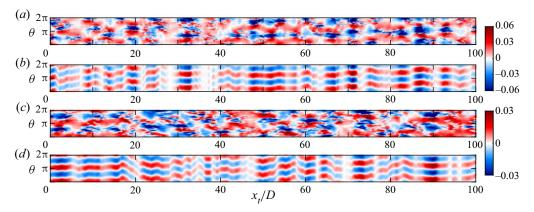
Figure 5. The  $u'_x$  field on a  $x_t/D - \theta$  plane at  $r/D \approx 2.0$ , for  $(a,b) x_0/D = 40$ , and  $(c,d) x_0/D = 80$ . In (a,c), m = 1 is removed, and in (b,d), only m = 2 is shown.
