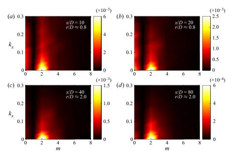
Figure 6. Two-dimensional power spectral density of the streamwise velocity fluctuation in  $k_x$ -m space, for: (a) x/D = 10,  $r/D \approx 0.8$ ; (b) x/D = 20,  $r/D \approx 0.8$ ; (c) x/D = 40,  $r/D \approx 2.0$ ; (d) x/D = 80,  $r/D \approx 2.0$ . The m = 1 wavenumber is removed so as to de-emphasize the VS structure.
