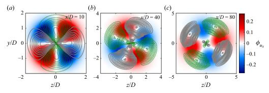
Figure 12. Leading SPOD mode of m = 2 and  $St \to 0$ , for (a) x/D = 10, (b) x/D = 40, and (c) x/D = 80. The false colours represent the real part of the streamwise velocity component  $\text{Re}[\phi_{u_x}^{(1)}(St \to 0)]$ , and the grey lines and green dotted lines correspond to positive and negative streamwise vorticity  $\text{Re}[\phi_{\omega_x}^{(1)}(St \to 0)]$ , respectively.
