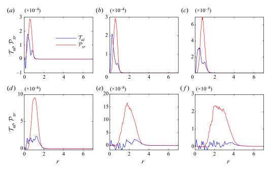
Figure 18. Nonlinear transfer ( $T_{nl}$ ) from the VS mode and the shear production ( $\mathcal{P}_{xr}$ ) at different streamwise locations for the m = 2,  $St \to 0$  mode, for (a) x/D = 2, (b) x/D = 3, (c) x/D = 5, (d) x/D = 10, (e) x/D = 40, and (f) x/D = 80.
