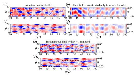
Figure 2. Instantaneous streamwise velocity on  $x/D-\theta$  planes at (a,b,e) r/D = 1.25 and (c,d,f) r/D = 2.5. Plots (a,c) show the full streamwise velocity field; (b,d) show the field reconstructed from the m = 1 contribution only; (e,f) show the field with the m = 1 contribution removed. Rectangular boxes in (e,f) emphasize the large-scale streaks in the flow field with the m = 1 mode removed.
