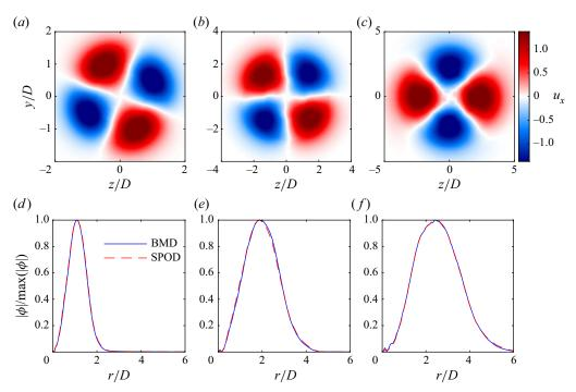
Figure 17. Cross-BMD modes for the triad [1, 1, 2] in azimuth and (0.135, -0.135, 0) in frequency, at three streamwise locations: (a) x/D = 10, (b) x/D = 40, and (c) x/D = 80. The false colours represent the real part of the streamwise velocity component. The absolute value of the BMD mode and the corresponding leading SPOD mode are compared in (d)–(f).
